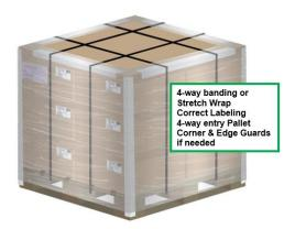
Band pallets through openings with plastic banding:
