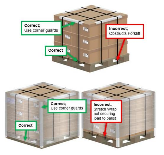
Stretch wrap pallet with several rotations around the base of the pallet:
