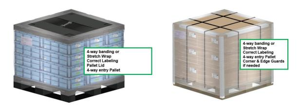
Band pallets through openings with plastic banding:
