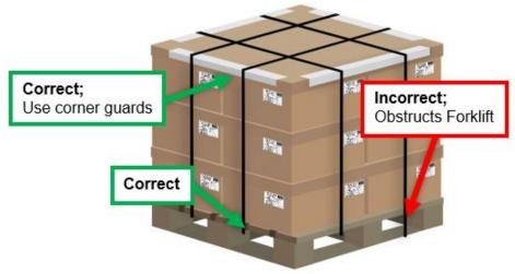
Stretch wrap pallet with several rotations around the base of the pallet:
