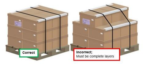
4.27.7 When corner supports are required for stacking strength, the preferred option is corrugated; Formed fiberboard angle boards, and roll ups. Wooden corner supports are an allowable alternative when heavy loads are applied. All wooden dunnage must follow the ISPM-15 specification.
