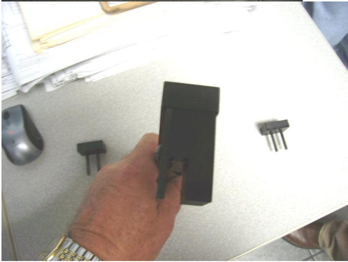
Hand held ISOWire True Position wire to each other (secondary call out)
